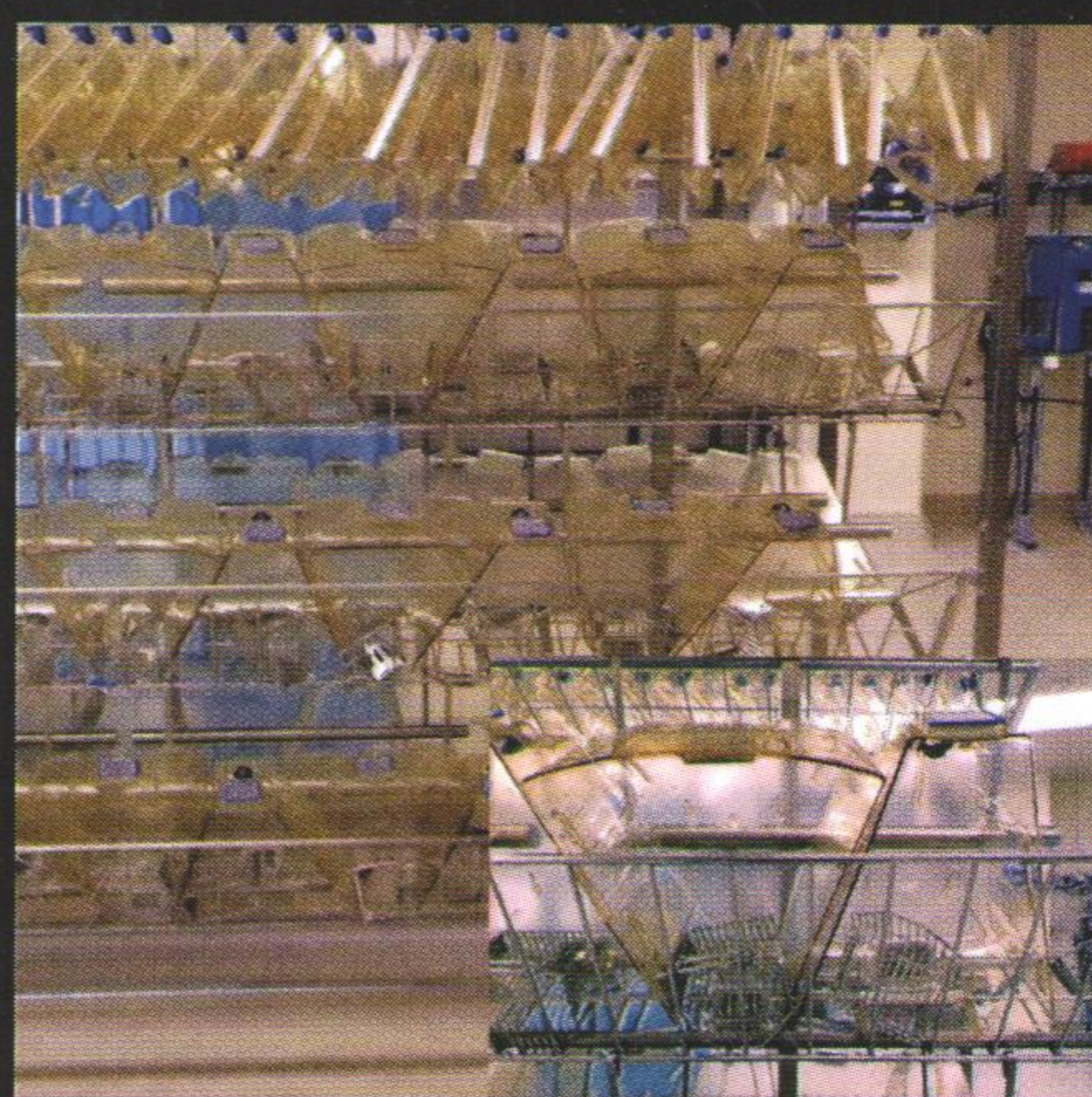
Figure 3. The lids are loaded on the top two shelves of the universal rack using one lid per slot. The lower 6 shelves are loaded with Optimice® cages. The feeders are loaded on the universal rack with the lid inside the cage (insert). This allows for efficient reassembly of the feeder within the cage after washing.
