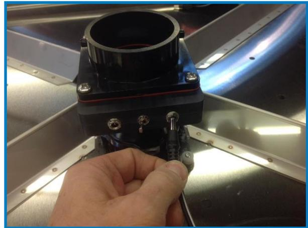
6. Flip the switch between the two power jacks to turn on the fan.
