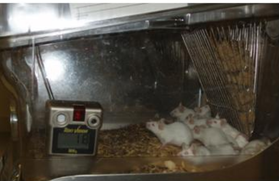
Cage Conditions: 19.5 °C, 29% RH, 18 ppm NH 3 15 weanies (6 weeks old); Bedding change 19 days ago
