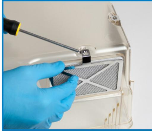
4. Push the filter components from within the cage to remove the coarse stainless screen and used filter medium. Discard the used filter medium.
