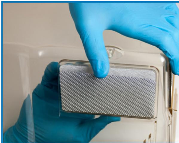
5. Place the new filter medium and then coarse stainless screen into the recess of the filter opening opposite the screw hole. The fine stainless screen **must** face the interior of the cage. If the screen positions are reversed, filter damage will result.
