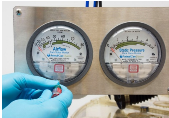
Figure 15: Zeroing the status monitor
