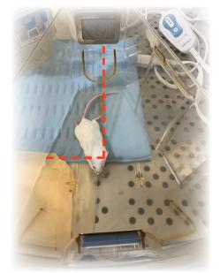
**Figure 4.** Heat elements of the electric heat blanket were positioned under the cage to occupy a similar configuration as the heat disk in the SMART system.
