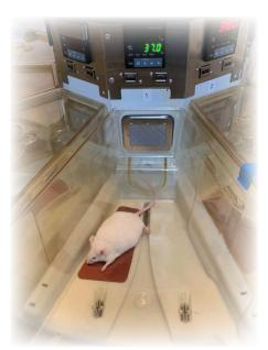
**Figure 3.** The SMART heat plate (red disk) occupies the left back quarter of the cage.
