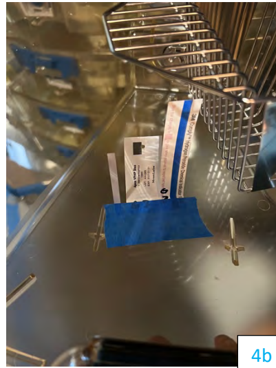
Figure 4a and 4b. Indicator placement. Images of chemical indicators outside the IVCs (4a) and biological and chemical indicators placed inside individual cages (4b).
