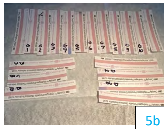
Figure 5a and 5b. Indicator results. Biological indicator (5a) and chemical indicator (5b) results following the hybrid hydrogen peroxide (HHP) cycle. Biological indicators show 6-log sporicidal decontamination in their purple color indicating no growth present, with the positive control in yellow confirming the integrity of the indicators. Chemical indicators show a pink color confirming the even distribution of HHP throughout the chamber and in individual IVCs.
