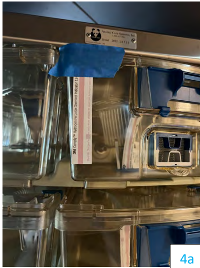
Figure 4a and 4b. Indicator placement. Images of chemical indicators outside the IVCs (4a) and biological and chemical indicators placed inside individual cages (4b).
