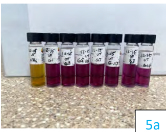
Figure 5a and 5b. Indicator results. Biological indicator (5a) and chemical indicator (5b) results following the hybrid hydrogen peroxide (HHP) cycle. Biological indicators show 6-log sporicidal decontamination in their purple color indicating no growth present, with the positive control in yellow confirming the integrity of the indicators. Chemical indicators show a pink color confirming the even distribution of HHP throughout the chamber and in individual IVCs.
