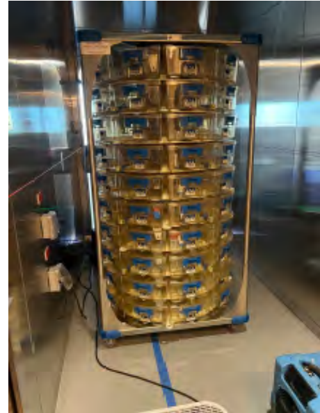
Figure 1. IVC rack with cages. Pictured is the circular IVC rack with washed IVCs in the chamber prior to decontamination.
